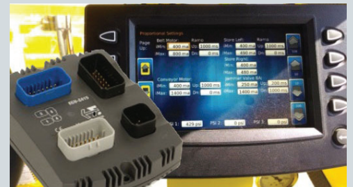
A HydraForce electronic controller (ECU-2415) provides CANBus control functionality, and a feedback loop for monitoring and troubleshooting all conveyor functions from the cab of the broom. Engine diagnostics, pump pressure, auger and belt operation, conveyor height and rotation and other performance parameters are all shown on a full color display screen.
