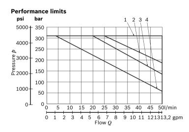
Lowest pressure setting curve for secondary valves
