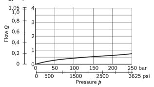
▼ Version: pressure drop  $\Delta p = \Delta p(Q)$  ( $P_{IN}$ -  $P_{OUT}$ ) to the next section psi bar
