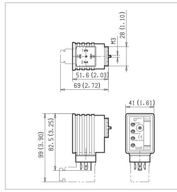
**Supply:** yellow LED, lit up with power ON. **Off Set:** minimum current adjustment. Adjust solenoid current so that the desired minimum value is obtained. Clockwise rotation increases current.
