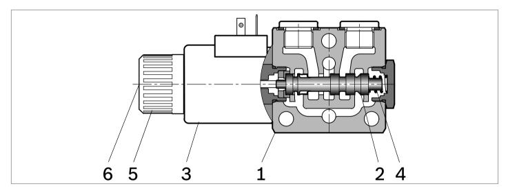
The sandwich plate design valve elements L808103P... are compact direct operated proportional solenoid valves which divert totally or partially the inlet P flow to Tank. These elements basically consist of a stackable housing (1) with a control spool (2), one solenoid (3), and one return spring (4).
