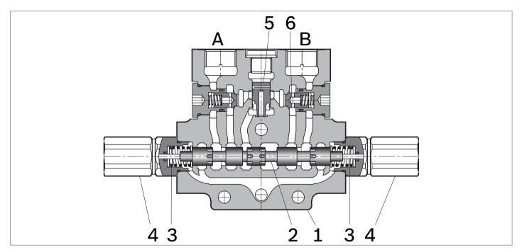
The sandwich plate design directional valve elements L85P5... are compact direct hydraulic operated pressure compensated proportional valves which control the start, the stop, the direction and the quantity of the oil flow, with FLOW SHARING principle. These elements basically consist of a stackable housing (1) with a control spool (2), two hydraulic operating blocks (4), and two return spring return (3).
