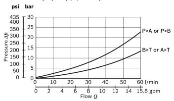
The curves refer to the spool fully open. Measured with hydraulic fluid ISO-VG32 at 45° ±5 °C (113° ±9 °F); ambient temperature 20 °C (68 °F).
