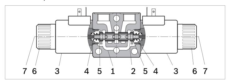
The sandwich plate design directional valve elements L8081... are compact direct operated proportional solenoid valves which control the start, the stop, the direction and the quantity of the oil flow. These elements basically consist of a stackable housing (1) with a control spool (2), one or two solenoids (3), and one or two return springs (4).
