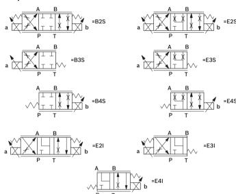
In neutral position, the valves cross section are as follows: E\_I  $\geq$  20% of nominal cross section.
