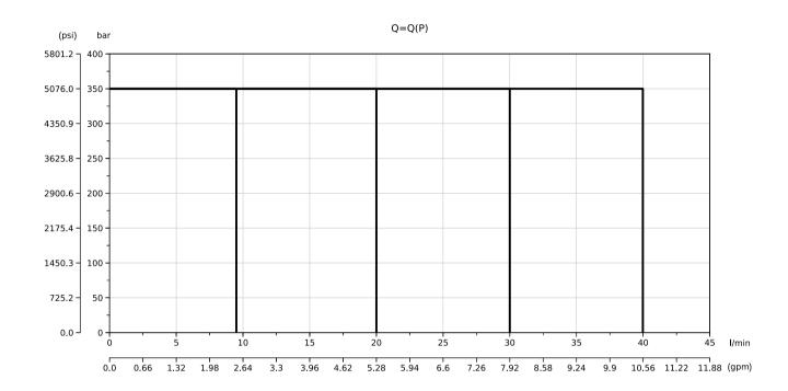
Measured with hydraulic fluid ISO-VG32 at 45°  $\pm$ 5 °C (113°  $\pm$ 9 °F); ambient temperature 20 °C (68 °F).
