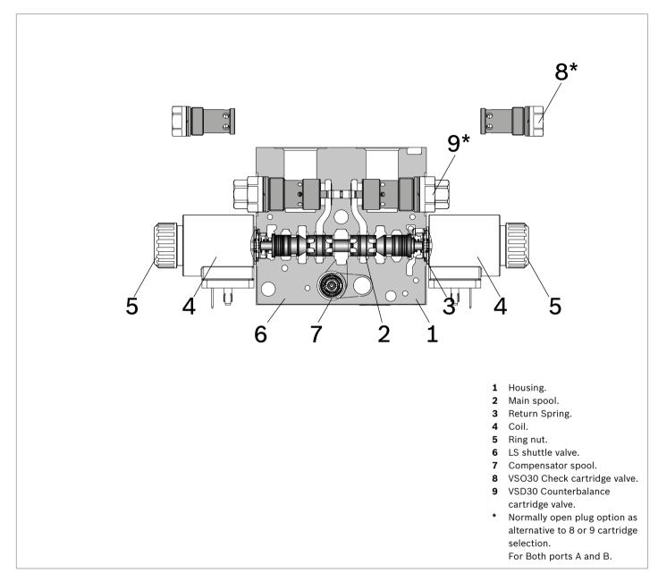
The EDG direct acting On-Off solenoid sectional valves with pressure compensation control the oil flow to actuators. These elements consist of a stackable housing (1) with a control spool (2), two solenoids (4), two return springs (3). Each solenoid (4), energized, displaces the control spool from its neutral-central position. When the spool is shifted, flow delivery starts and is controlled by a 2 way pressure compensator (7) (P > A; P > B).
