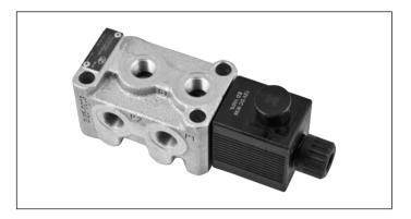
Series 01 Maximum operating pressure 310 bar (4500 psi) Maximum flow 60 l/min (15.85 gpm) Ports G 3/8 - G 1/2 - SAE8
