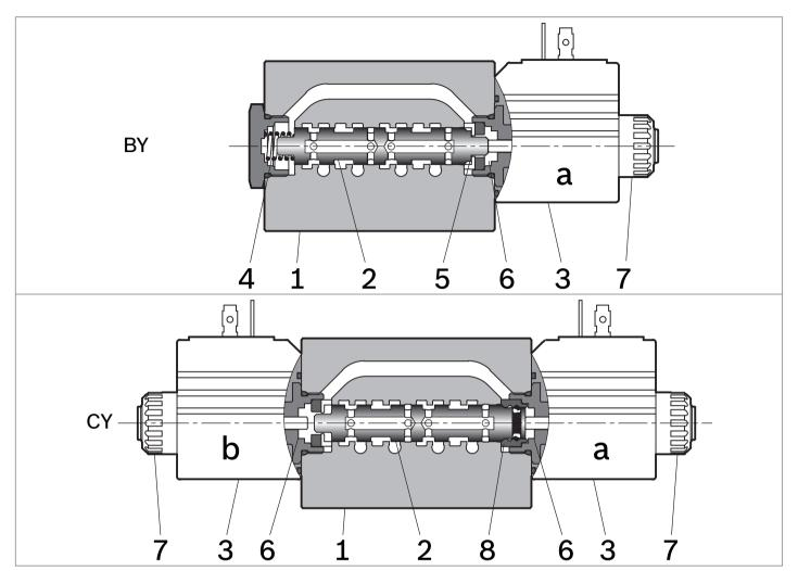
A valve basically consists of a housing (1), a control spool (2), one or two solenoid (3), and a return spring (4).
