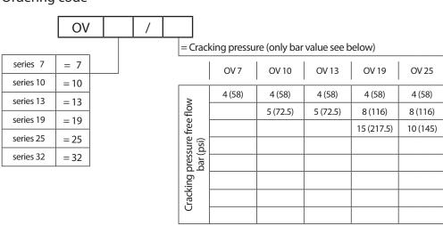
Do not specify for the standard pressure 0.5 bar (7.25 psi) Note: The OV32 cracking pressure is 0.5 bar (7.25 psi)
