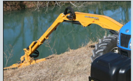
The Alamo Maverick™ Mower reduced cylinder drift during boom extension with HydraForce cartridge valves.
