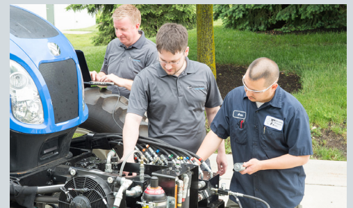
Running diagnostics on the main manifold is made easier with EVDR controllers, since you can adjust parameters right on the machine.
