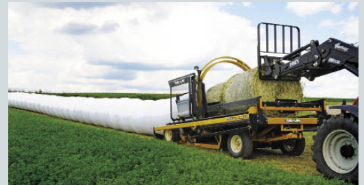
The Tubeline ECV bale-wrapping machine now uses the power of proportional control to wrap bales right in the field.
