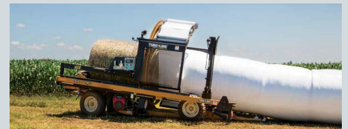
Proportional control allows "soft-starting" the wrapping function to prevent the plastic from tearing. The priority-on-demand hydraulic circuit uses a HydraForce EC16-42 pressure compensator and a PV70-33 proportional flow control valve.
