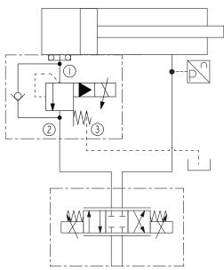
Using a pressure control for lowering is comparable to using a counterbalance valve. With a counterbalance valve, pressure in the base end of the cylinder is a fixed ratio above pressure in the rod end. Whereas when using the EHBL, the pressure sensor on the rod end monitors resistance to movement, allowing the pressure control to dynamically adjust the base end pressure maintaining stability.
