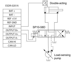
When used with a position sensor integrated to the cylinder, the ESDR can control its position. The PID loop can be tuned to match the desired response. For example it can be optimized for speed, or to minimize overshoot/overcorrection. The simplified circuit shows an SP10-58D proportional directional valve with motor spool. An isolated load sense signal communicates the load pressure to the load-sensing pump. A stroke sensor with analog output forms the feedback leg of the PID control.
