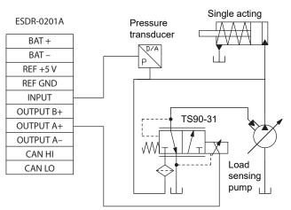
You can control the force of a press, grapple, or other clamping device using a proportional relief valve with a pressure sensor to communicate the load to the ESDR. In the example, the ESDR regulates a load-sensing pump using a TS90-31 to control the load-sensing pressure. This achieves force control of the single-acting cylinder.
