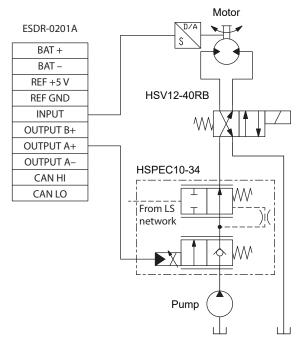
The ESDR can provide closed-loop motor speed control when used with a speed pickup that provides an analog output. In the example an HSPEC10-34 provides pressure compensated flow control and an HSV12-40RB can reverse the direction of rotation as needed possibly to clear the radiator in a fan drive application. The main vehicle control can close the loop on engine temperature. This example can also drive a conveyor or auger to provide closed-loop control of product feed rate.
