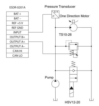
In another variation of force control, you can easily control the torque of a hydraulic motor with a proportional relief valve, using a pressure sensor for feedback. In the example, the ESDR controls a TS10-26 proportional relief valve. An HSV12-20 is
