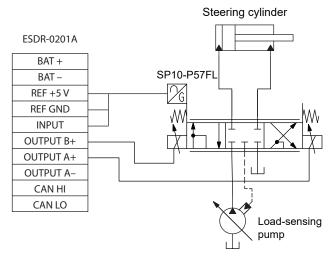
For applications such as auto-steering where precise and repeatable flow control is needed, you can use the ESDR with an LVDT position sensor that feeds the spool position back to the 0-5 V input. In this simplified example, the SP10-P57FL (patent pending) controls flow to the double-acting steering cylinder while providing an isolated load-sense signal back to the pump.
