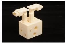
3-D printing can be used to determine fit and footprint for your HydraForce hydraulic control solution.
