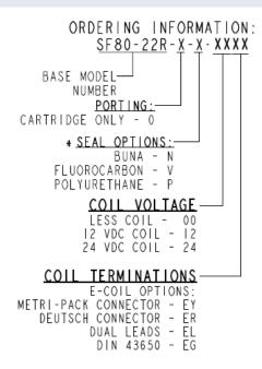
POLYURETHANE SEALS RECOMMENDED FOR OPERATING PRESSURES ABOVE 3500 psi [241 bar]
