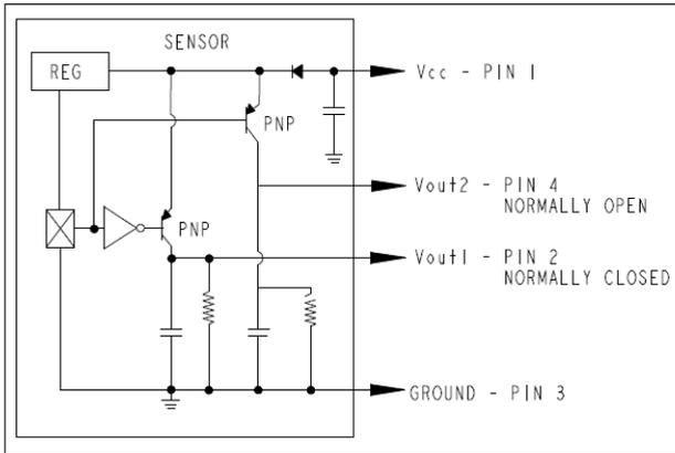
N3 SENSOR WIRING DIAGRAM
