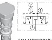
A screw-in, cartridgestyle inverted shuttle valve, which can be used to help protect against brake or steering failure in the event of loss of pressure in either one of two accumulators.
