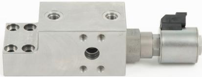
**ALL IN ONE** - The EBLV boom lock valve is an integrated assembly that features a proportional pressure control cartridge valve in a single-piece housing that also contains a check valve.
